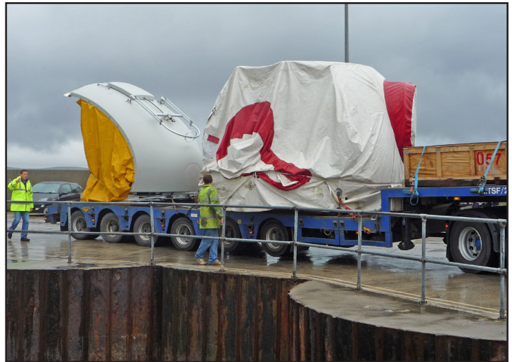
Pictured right: Offloading part of the turbine August 2009
